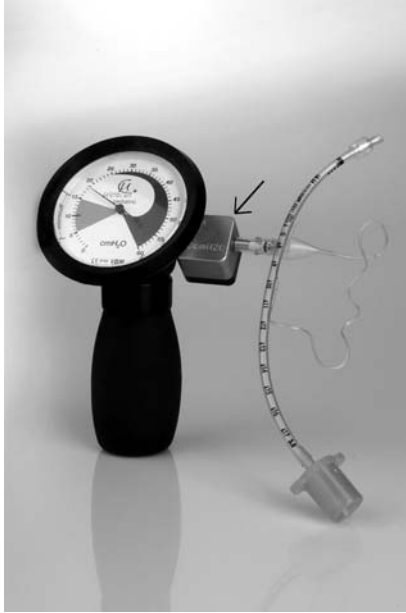
Fig 1 Test assembly used in the cuffed group: cuffed paediatric TT (Microcuff® PET) attached to a cuff pressure manometer with pressure release valve (arrow) limiting cuff pressure at 20 cm H 2 O.
